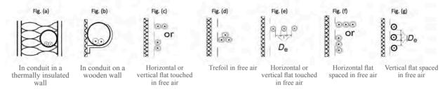
**Laying Conditions:** Ambient air temperature of 40 °C and ambient ground temperature of 35 °C. In case of different laying conditions, appropriate correction (derating) factors have to be applied to cater for the actual installation conditions.
